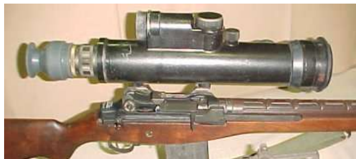
AN/PVS-1 Night Vision Sight "Starlight Scope" (1 st Generation) used on M14 Rifle (circa 1965-70)
